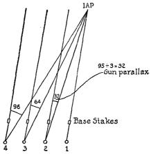
FIGURE 44.-Laying guns on parallel lines
