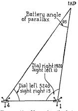
FIGURE 43.—Measuring the battery angle of parallax
