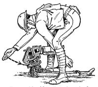
FIGURE 36.—Mounting the tripod
