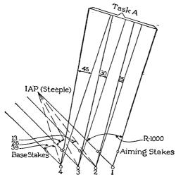
FIGURE 48.—Establishing base and direction lines
