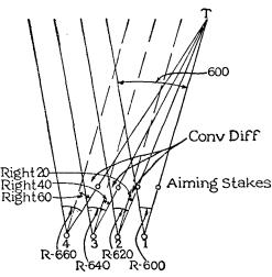
FIGURE 47.—Laying guns on a narrow or point target
