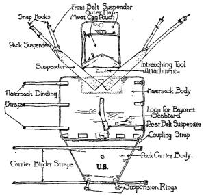
FIGURE 84.-Haversack with pack carrier attached
